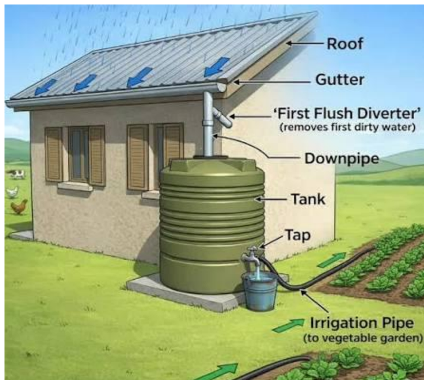
Picture 3: Harvesting rainwater from a sloping roof into a tank
